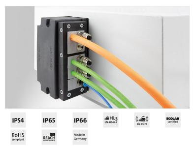
KEA 24 is a cable entry adapter for accommodating various icotek cable entry frames and plates of size 24. The adapter allows cables to be routed at a 90° angle. The installation direction can be horizontal or vertical. The cables are protected against mechanical tension in the entry and exit areas. Wall mounting is done either with screws and nuts or by using threaded bushings. A suitable wall seal is included in the scope of delivery. icotek also offers suitable punches for the cut-out.
